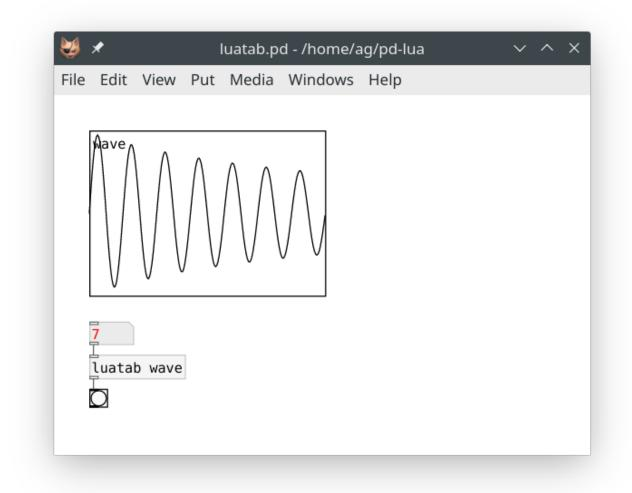
In the same vein, the Pd-Lua distribution includes a much more comprehensive example ltabfill.pd\_lua, which leverages Lua's load function to create a waveform from a user-specified Lua function created dynamically at runtime (instead of being hard-coded into the Lua code, which is what we did above).
