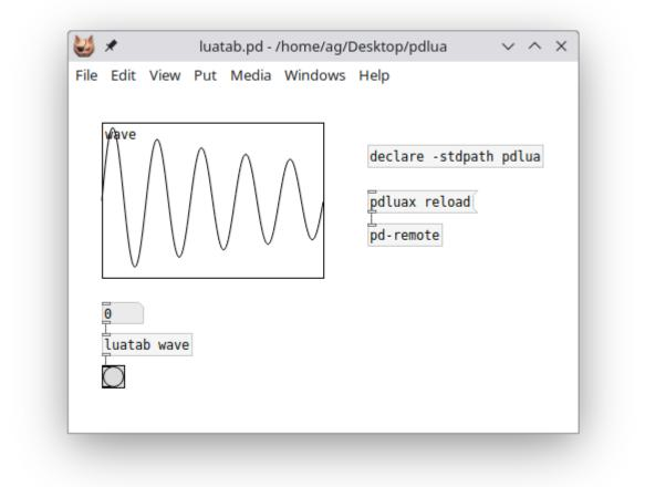
**NOTE:** To make Pd find the pd-remote.pd abstraction without having to copy it to your project directory, you can add the pdlua external directory (which is where the abstraction gets installed) to your Pd library path, either in your Pd setup, or inside the patch with a declare -stdpath object, as shown above.
