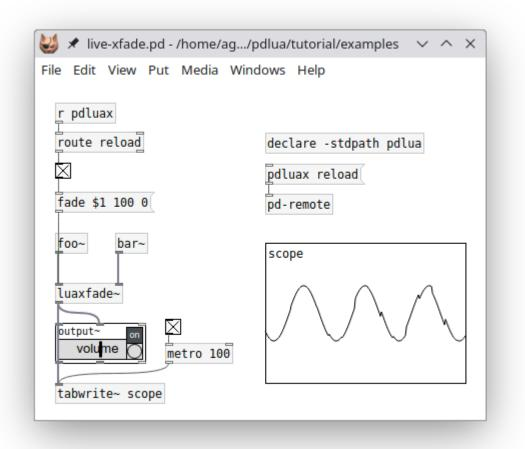
The foo~ and bar~ objects in this example are essentially the same, with some minor variations in the sound generation parameters. The particular sounds in this example are not important, each object just outputs a random walk of sine waves of varying frequencies with some phase distortion. But they *will* produce clicks when switching them abruptly, thus we need a smooth cross-fade between the two sound sources. This is handled by the <u>luaxfade</u> object from the Signals section.
