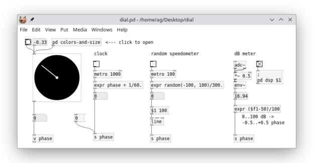
The extended example adds messages for resizing the object and setting colors, and also shows how to save and restore object state in the creation arguments using the set\_args() method mentioned at the beginning of this section. The accompanying patch covers all the examples we discussed here, and adds a third example showing how to utilize our dial object as a dB meter.
